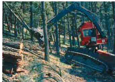
A feller-buncher severs trees and lays them in bunches with limbs and tops attached. Bunches are oriented with tree trunks facing downhill.
